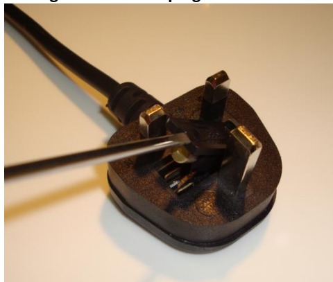
Figure 28: Mains plug fuse removal
