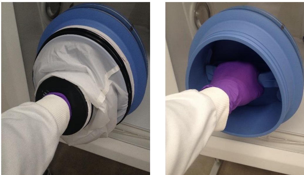
Figure 14: Arm inserted into Ezee-Sleeve (Shown with and without Ezee-Sleeve)
