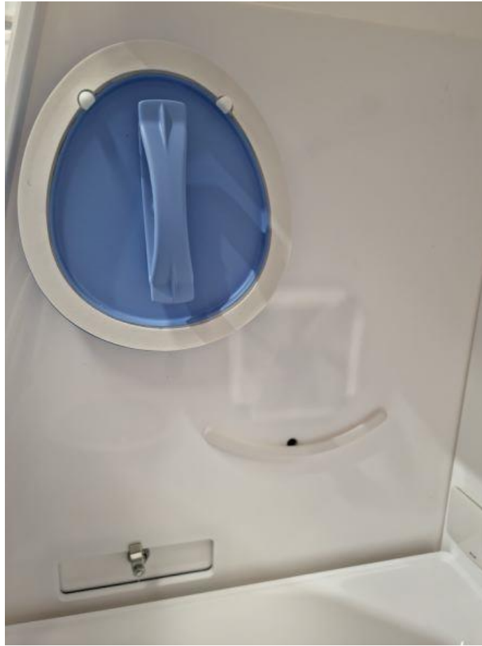
Figure 19: Glove port cap storage location inside workstation
