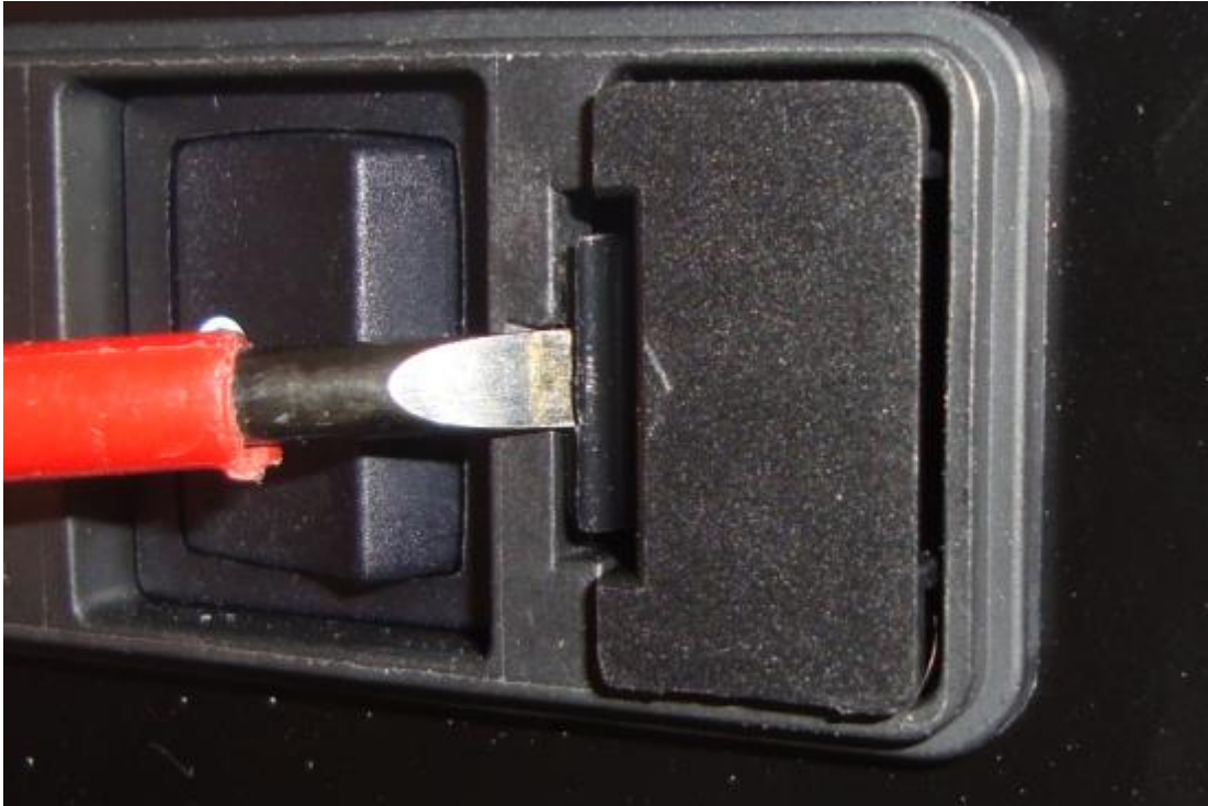
Figure 29: Mains fuse holder removal
