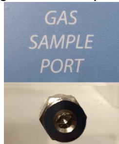
Figure 25: Gas Sample Port
