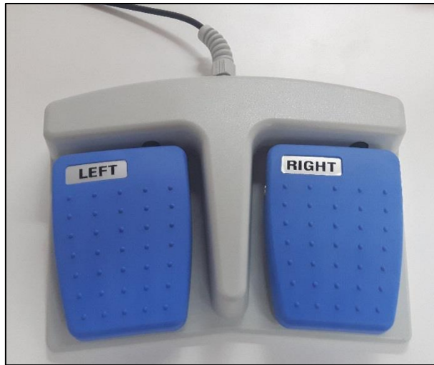
Figure 15: Foot pedals for right and left glove ports
